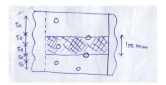
c. Determine the design tensile strength of the plate 130mm\*12 mm with the holes for 16 mm diameter bolts as shown in fig. Steel used is of Fe410 grade quality.
